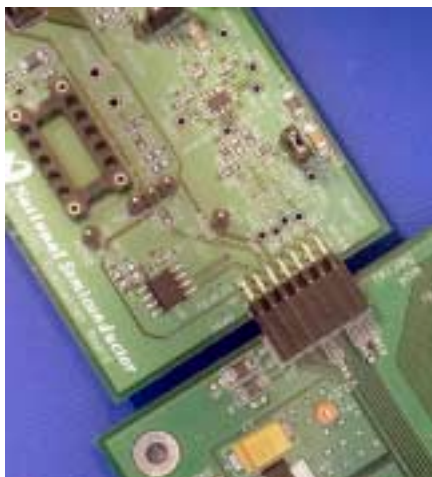
Figure 6: WV4 to ADC121C02XEB Connection
